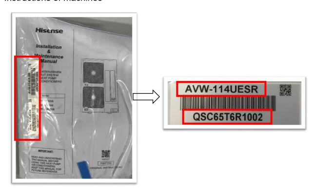
Attention: The machines type and serial number must be identical
